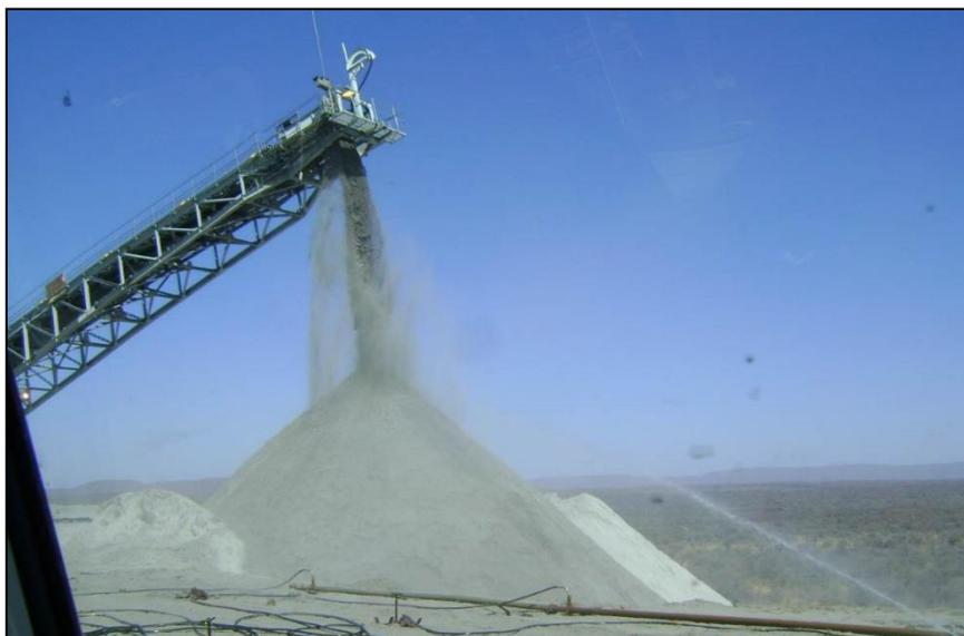
**Figure 13: Moisture condition (typically 10%) of ash at arrival at the ash facility (Matimba Power Station)**
